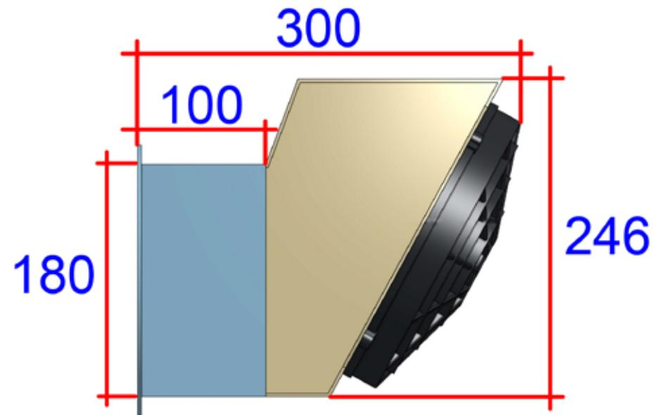
Vessel cut out (penetration) size = 700mm Wide x 180mm High
